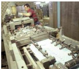
(Left) Furniture manufacturers use vacuum in place of traditional clamping methods to avoid damage.
